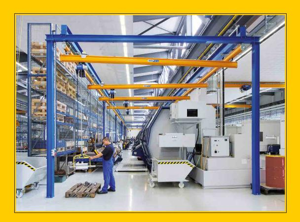
Bespoke support structures for fixing light crane systems
