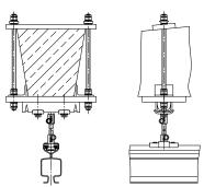
Embracing brackets clamp around the building trusses so that drilling completely through them is not necessary.
