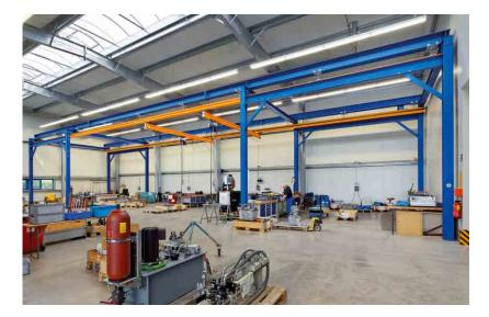
Individually tailored portal structures offer solutions, for instance, when the ceiling structure is unsuitable for supporting an HB crane system. There are free-standing versions as well as those connected laterally to the building structure.
