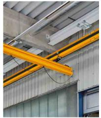
Auxiliary girders provide additional hanging positions for the suspension of the HB crane installation. They are fixed directly between building girders, enabling even large distances to be bridged.
