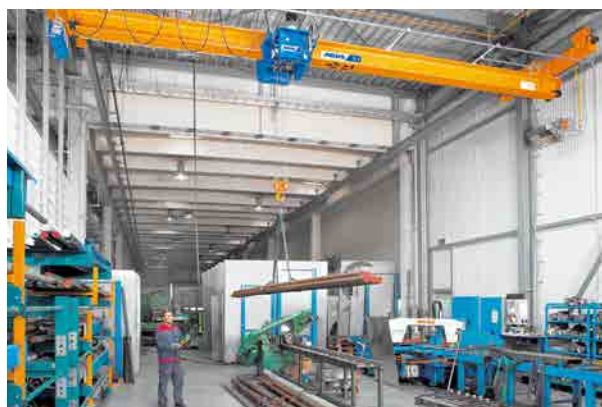
Type E monorail hoist on a type EDL underslung overhead travelling crane
