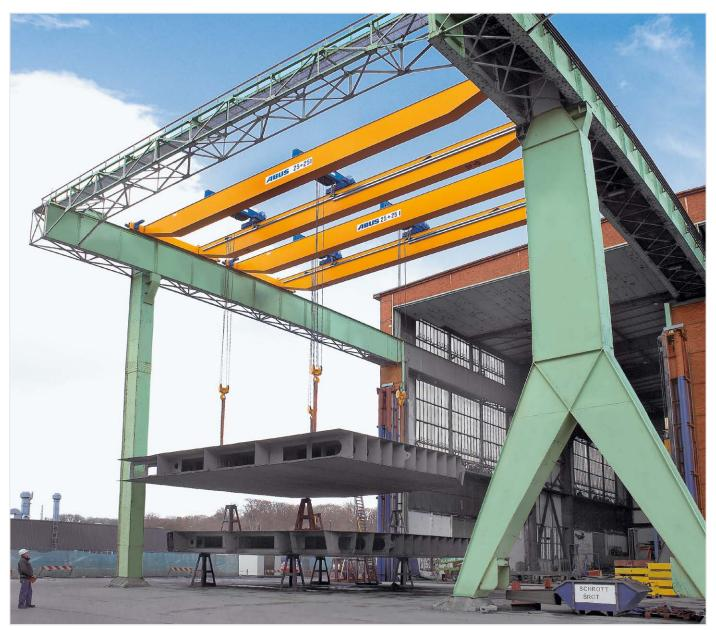
ABUS tandem control offers a professional solution for this particular logistical challenge. It makes it possible to move two cranes simultaneously via remote control. The operator is able to select the optimal
