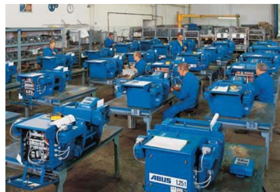
Assembly of monorail hoists
