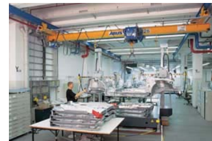
Type E monorail hoist on a type EDL underhung overhead travelling crane
